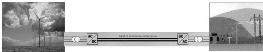
Figure 8 Schematic diagram of a HVDC Light transmission for wind power
